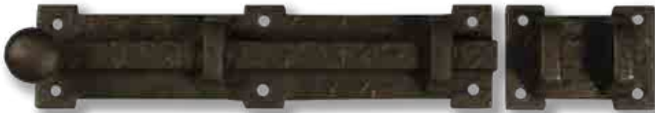
70-300 - Shutter Slide Bolt 6-1/2" x 1-1/2" Catch 2" x 1-1/2" Throw 2"
